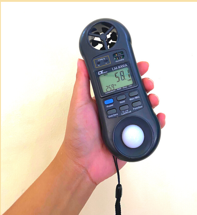
Image 54. Tool used in measuring air quality (Anemometer, %RH, Temperature, Lux) (Source: Photo taken at ATI-ITCPH, 2022)
